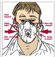
7 Before entering the workplace, a user seal check should be carried out. This is done by placing your hands over the filter material and breathing in. The mask should suck down onlo your face when you breathe in sharply. You should hold your breath for ten seconds and the disposable respirator should not loosen. If it does, you should readjust
